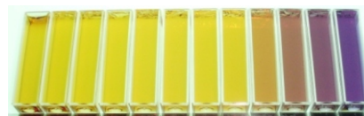
Figure 16. Optical dose responses to gamma radiation, photon and electron clinical beams of FXG solution
