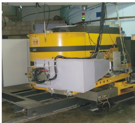
Figure 1. The neutron powder diffractometer 'Aurora'
