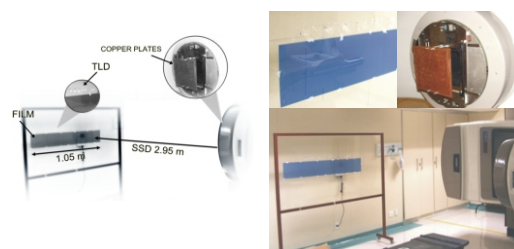
Figure 1. Experimental configuration for TSET dose distribution measurements using TLD and radiochromic films
