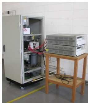
Figure 13. 1kW PEMFC system made with IPEN technology
