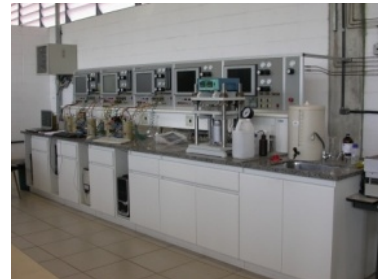
Figure 14. New test benches improved their previous versions by the inclusion of mass flow meters and a PLC controller
