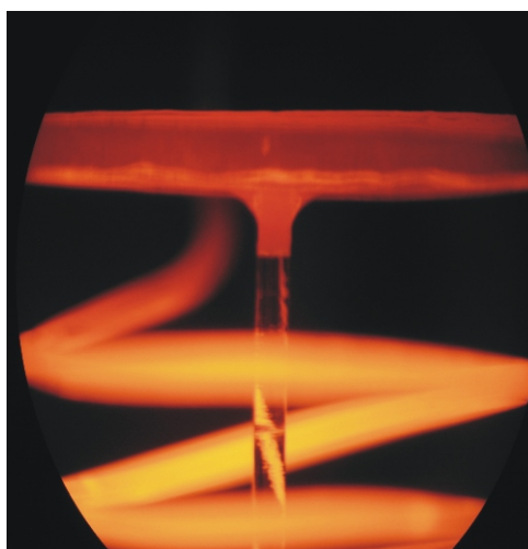
Figure 1. \text{BaLiF}_3 single crystal fiber growth
