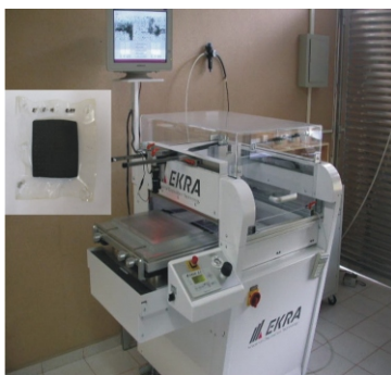
Figure 1. Sieve-printing apparatus for Membrane-Electrode-Assembly (MEA) production
