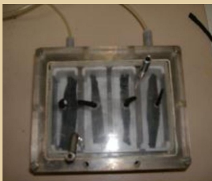
Figure 3. A 4-stage electrolytic cell with ion exchange electrodes used in the treatment of wastes containing Cs or Cr
