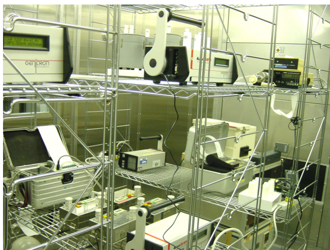
FIG. 3. Inside view of the radon/aerosol chamber at the 1st inter-comparison experiment at the NIRS
