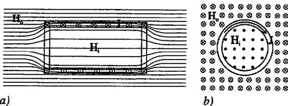
Figure 1: Shielding effectiveness of a cylindrical shield
