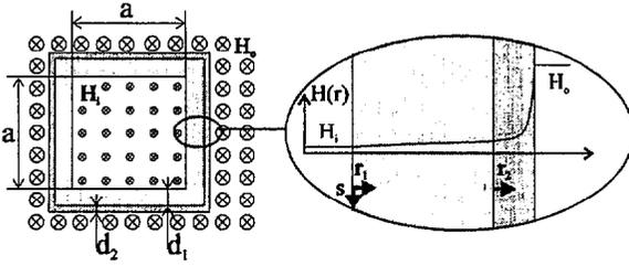
Figure 6: Magnetic field in a coated enclosure
