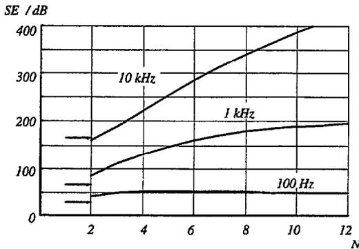
Figure 12: SE of a cylindrical enclosure consisting of N shields of copper
