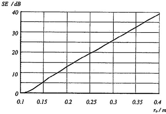
Figure 10: Difference of the SE of a doubly shielded and a single shielded cylindrical enclosure.
