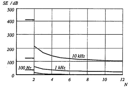
Figure 13: SE of a cylindrical enclosure consisting of N shields of magnetic material
