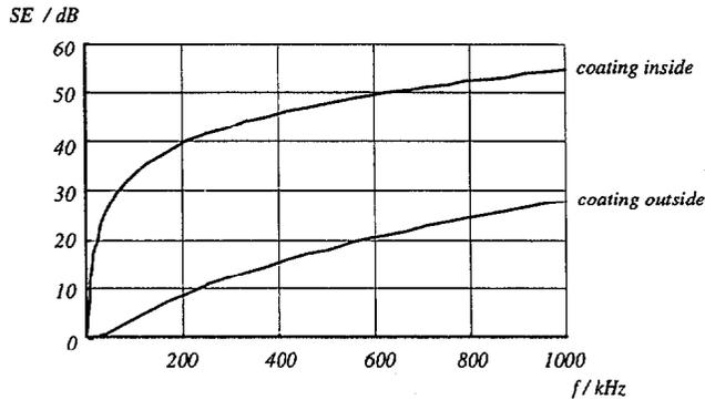
Figure 8: SE of an enclosure with a magnetic coating
