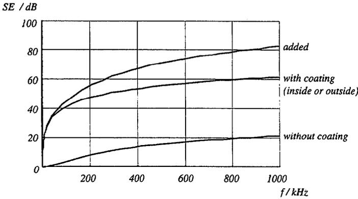
Figure 7: SE of a coated enclosure according to Figure 6
