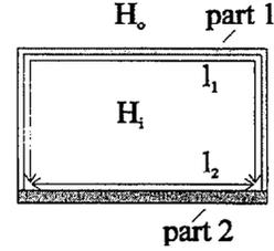
Figure 3: Shield with different wall properties
