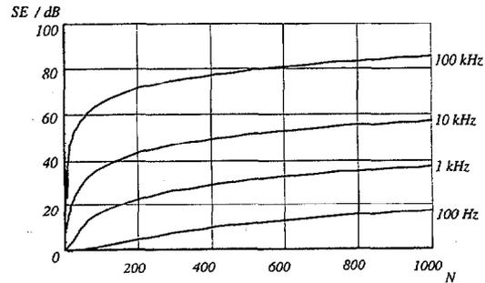
Figure 17: SE of the cylindrical enclosure of figure 15, made of magnetic material, depending on the number  $N$  of cavities
