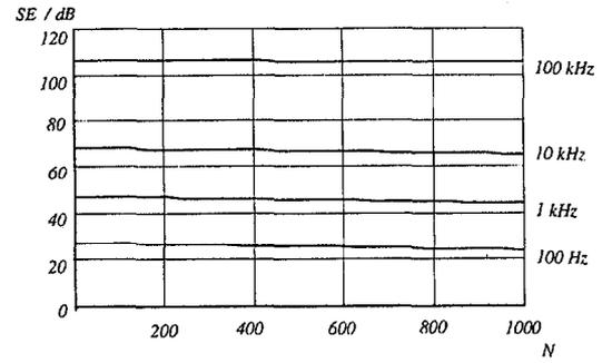
Figure 16: SE of a cylindrical copper enclosure of figure 15, depending on the number of cavities
