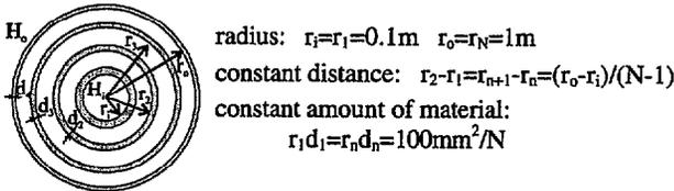
Figure 11: Cylindrical enclosure consisting of N shields
