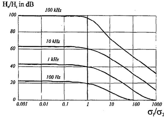
Figure 4: Shielding effectiveness of a quadratic shield with different wall properties, depending on the conductivity  $\sigma_2$  of the bottom
