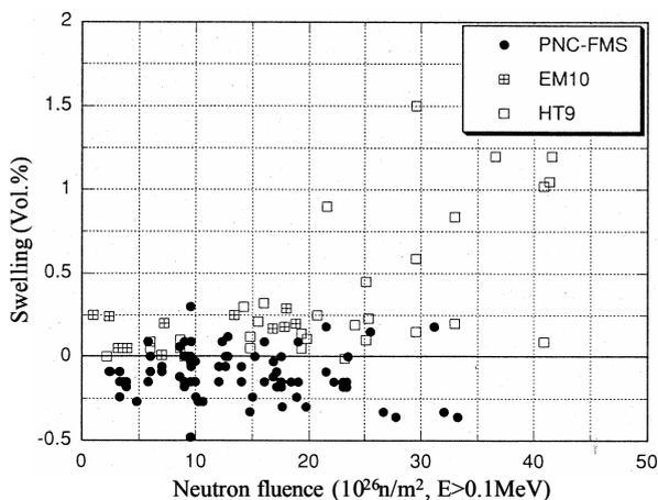
Fig. 4 Swelling of Ferritic Steels (384-688°C)
