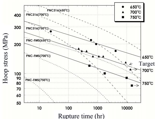
Fig. 5 Creep Rupture Strength of ODS Ferritic Steel (In air)
