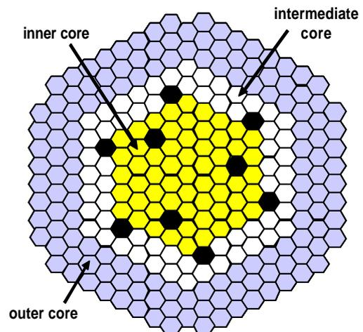
Fig. 2 500MWe 3 region(individual fuel pin diameters) core configuration
