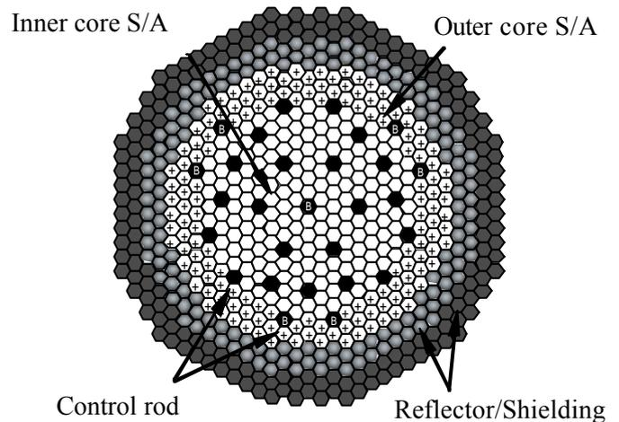
**Fig. 1** Core configuration of 750MWe MOX fuel core
