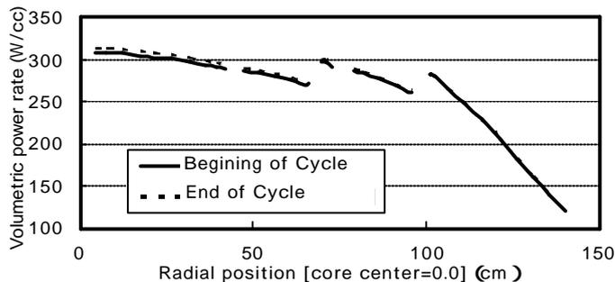
Fig. 3 Radial Power Profile of Core in figure 2
